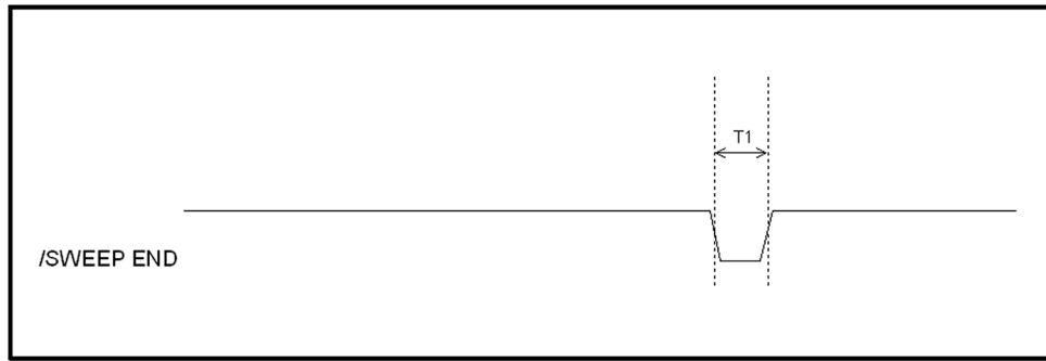
Figure C-3 Pulse width of /SWEEP END
